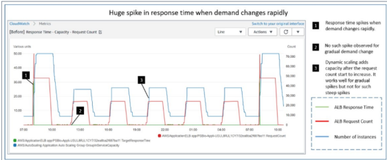
Fig. 2. CloudWatch Metrics Showing Latency Spike Due to Rapid Load Increase
