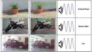
The proposed system successfully detected the objects which are far away in the outdoor environment with good accuracy. Following are the objects that are detected in the outdoor environment. The system was successful in detecting the objects which were more than ten meters away in the outdoor environment.
