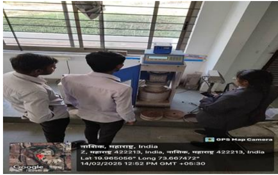
Figure 6: - Cube under compressive testing machine
