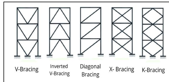
Fig 1 Bracing Details
