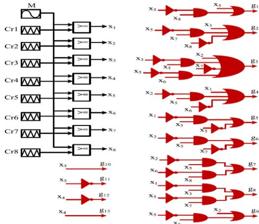
Fig. 4b. Gate signal pattern for triggering the switches
