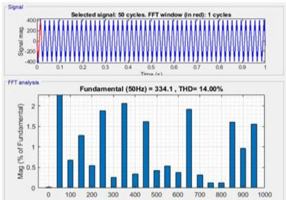
Fig.6a Output voltage
