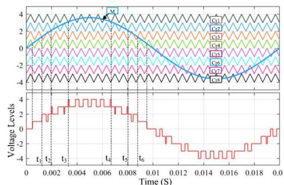
Fig.4a. Level Shifted Pulse Width Modulation.
