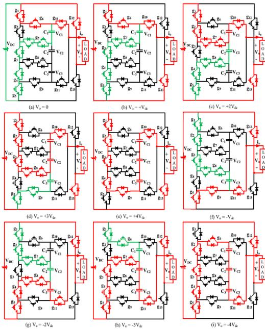
Fig.3 Operating modes of the proposed nine-level output voltage topology
