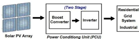
Fig.1 Schematic structure of the two-stage PV system
