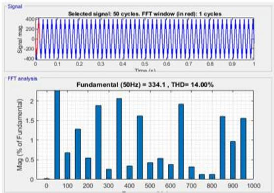
Fig.5d THD plot of the output voltage
