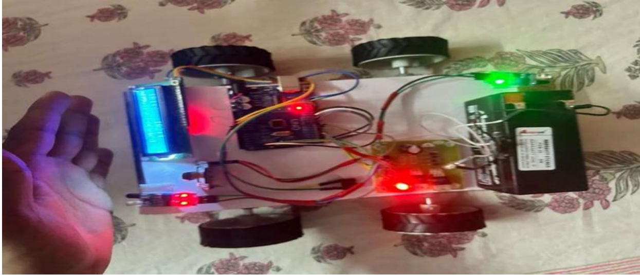
Fig.3: Buzzer Activates when obstacle is Detected and LED get activated
