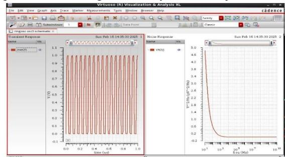
Fig :4.4 transient response and noise response of 5-stage SDRO
