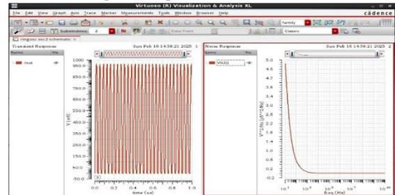
Fig :4.3 transient response and noise response of 3-stage SDRO
