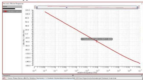
Fig: 4.2 PHASE NOISE OF 5-STAGE
