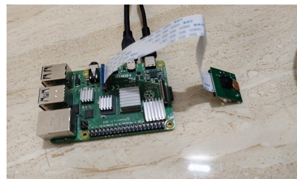
Fig. 2. IOT Device for Detecting leaves Diseases in Plants by Image Processing
