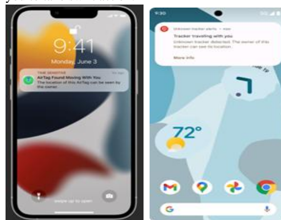
Figure 5: Alert displayed when unknown trackers are detected.
