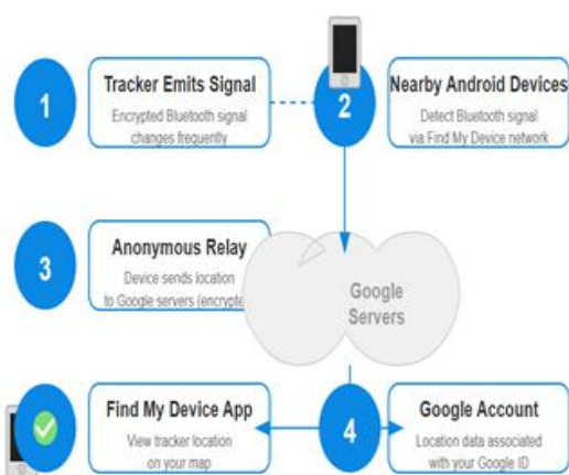
Figure 4: Illustration of how Android smart tags track location.
