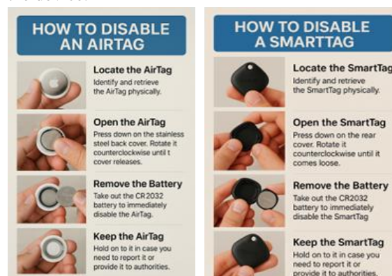
Figure 9: Example of the steps to disable an AirTag/Android Tag.
