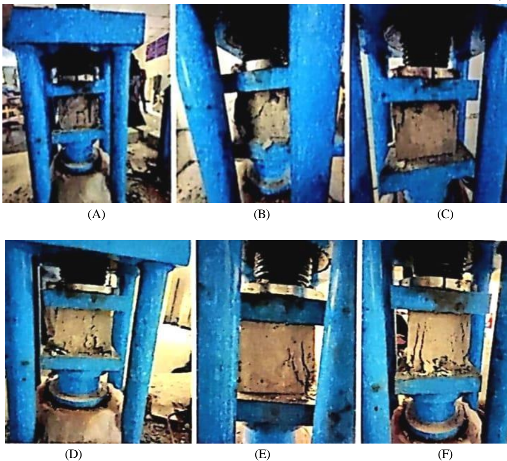
Fig 11. Compressive Strength Test on Concrete Cubes
