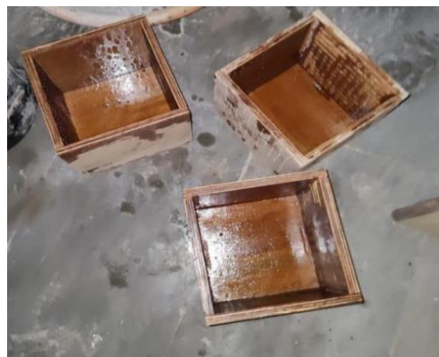
Fig 4. Wooden Mold (150X150X150 mm)
