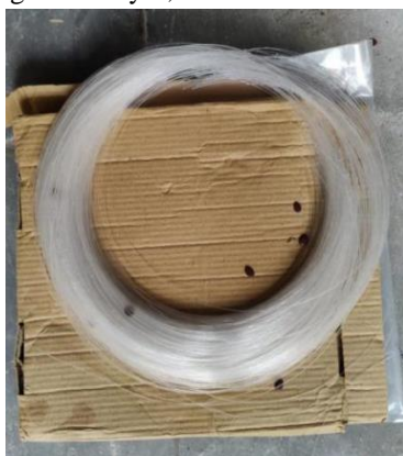
Fig 3. Optical Fiber (0.625 mm)
