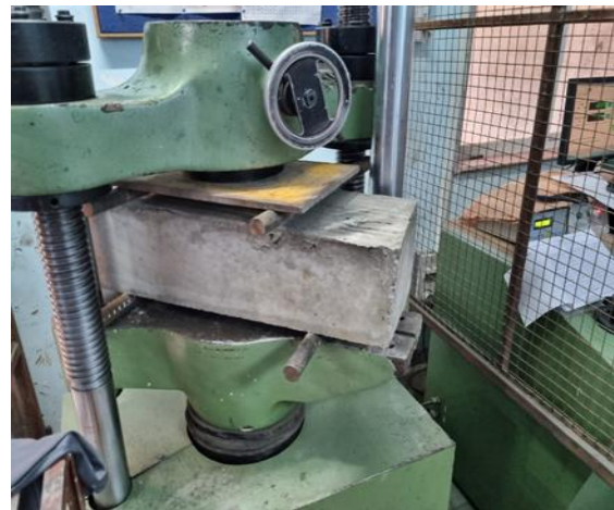
Fig.2 Setup in UTM with specimen
