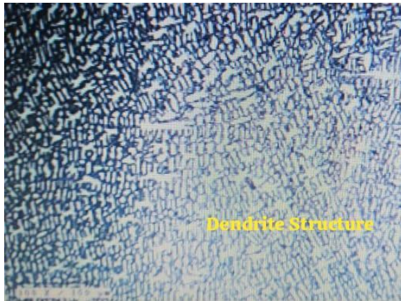
Fig 4.7: Weld – Mag: 100x
