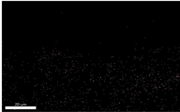
Fig 4.21: EDS Sodium (Na) distribution map
