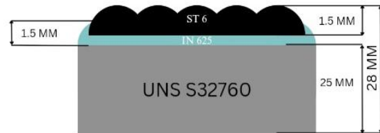
Fig. 3.1: Weld Model Diagram
