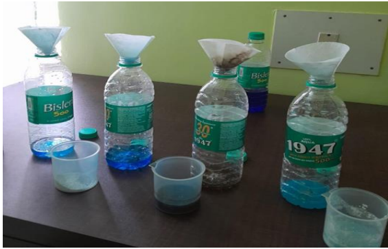
Fig 1. Filtering of the solutions with the respective adsorbents using filter paper.
