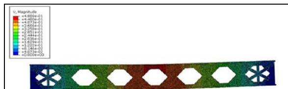
Finite Element analysis in cyclic load condition VS deflection (Case-1)
