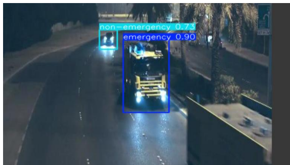
Figure.2. Emergency Vehicle Detected With Accuracy of 0.90
