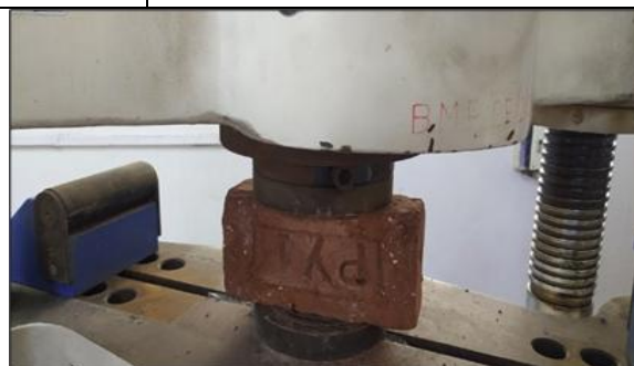
Fig.3 Compression Test on (UTM)
