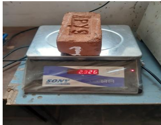
Fig.1 Water absorption test
