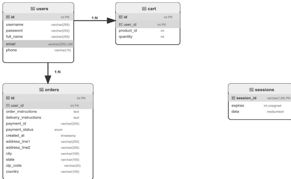
“Fig. 11” Schema design of backend
