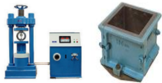
Figure 1: Compression Testing Machine (CTM) – used for evaluating compressive strength.
