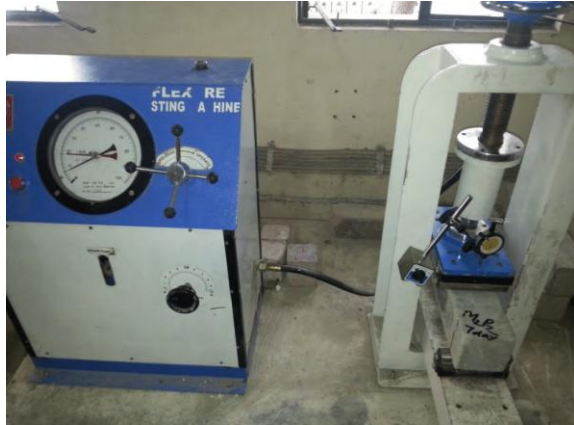
Figure 3: Flexural Testing Setup – used for modulus of rupture determination.
