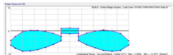
Fig.5: Variation of Stresses at Stage 6 - SDL from Super-Structure
