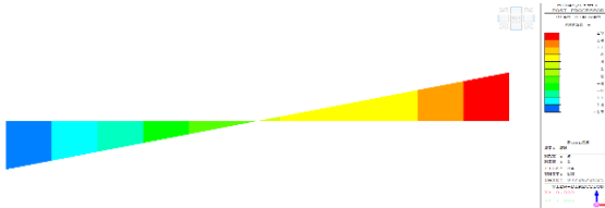
Fig 17: Shear force Diagram for Case 5-B4 Beam with Concrete Jacketing, External Prestressing and Minimum Reinforcement for Self-weight. (kN)
