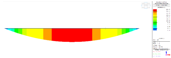
Fig 6: Bending Moment for Case 2-B1 Beam with Concrete Jacketing and Minimum Reinforcement for Self-weight. (kN)
