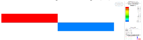
Fig 14: Shear Force for Case 4-B3 Beam with External Prestressing for Prestress. (kN)
