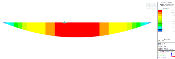
Fig 12: Bending Moment for Case 4-B3 Beam with External Prestressing for Self-weight (kN)
