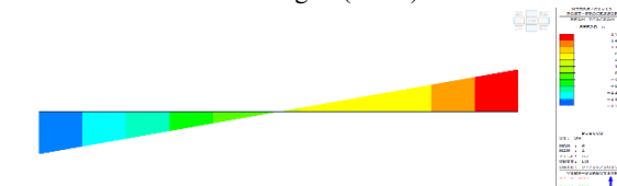
Fig 10: Shear Force for Case 3-B2 Beam with Concrete Jacketing and Maximum Reinforcement for Self-weight (kN)
