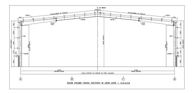
The following sections are illustrate the structural framing for a steel building, specifically the rigid frame cross sections along designated grid lines. These frames represent the primary load bearing structure of the building, designs to support roof loads, wind loads and other lateral forces.
