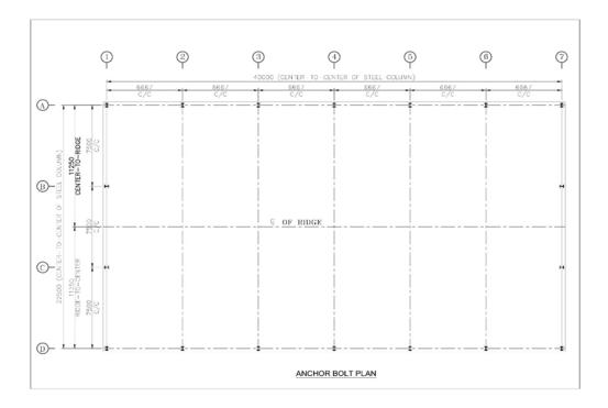
This image shows that proper alignment and accurate placement of structural elements during construction. The anchor bolt plan is a critical component of structural steel detailing. It specifies the exact location of anchor bolts which are used to secure steel columns to the concrete foundation.
