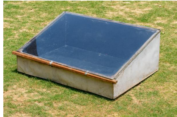
Figure 2: Photograph of the Fabricated Solar Still
