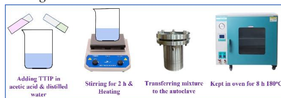
Fig. 1. Synthesis of TiO 2 by hydrothermal rout.
