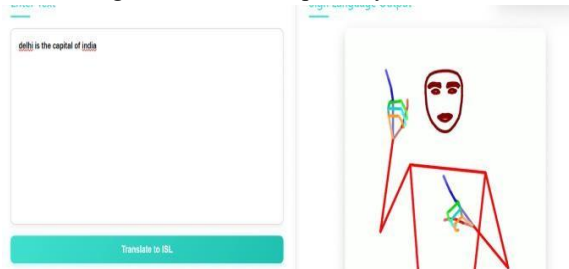
Fig.7: shows the stickman model performing ISL gestures using concatenated and smoothed. pose sequences.
