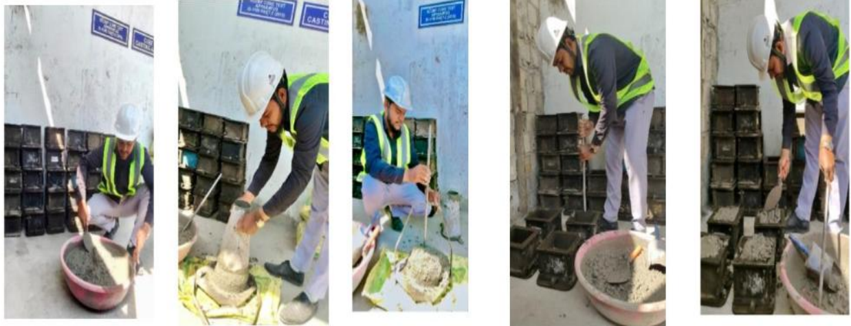
Fig 3. Checking Slump & Casting Cubes
