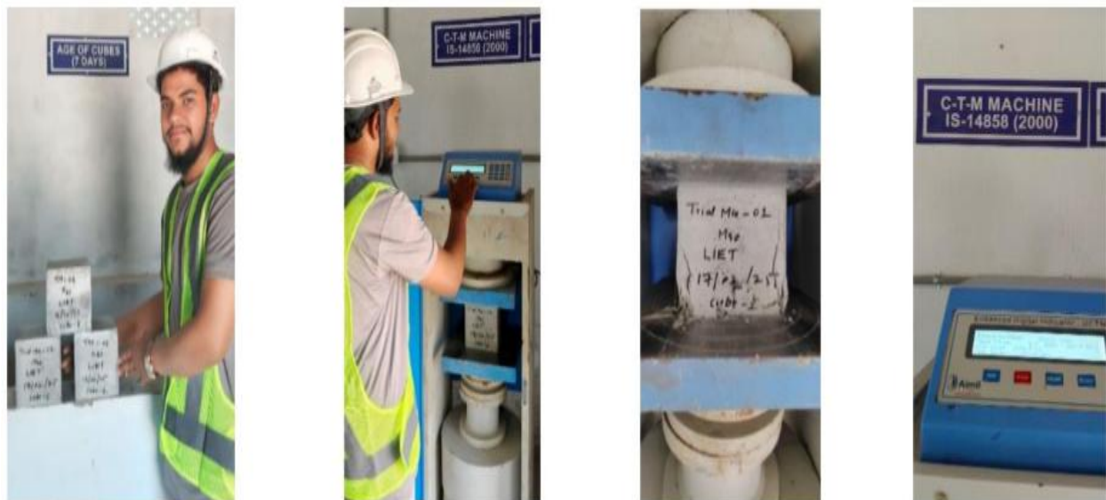
Fig 5. 7Days Cubes Strength Testing
