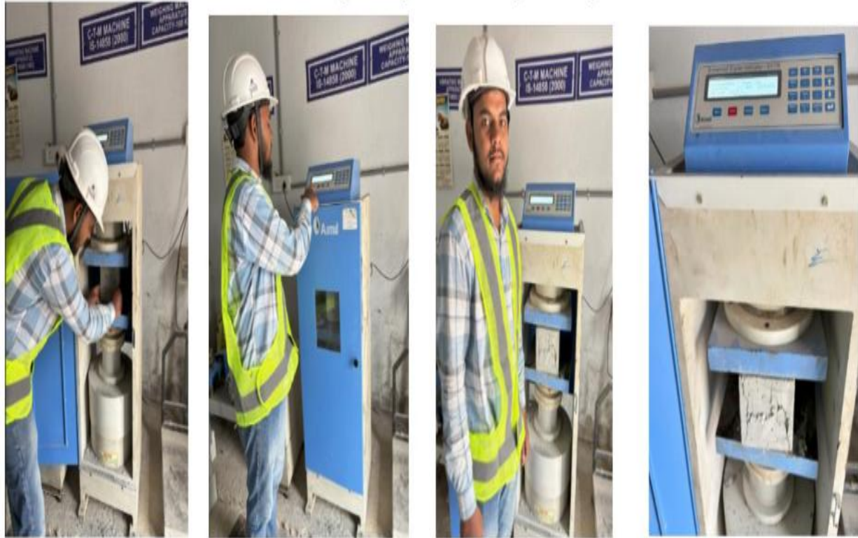
Fig 6. 28Days Cubes Strength Testing
