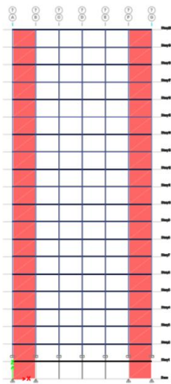
M15SP10°15 storey model with stepback and 10° slope with shear wall
