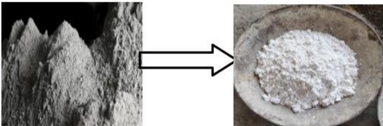
Figure 2: Partial replacement of cement with Lime sludge
