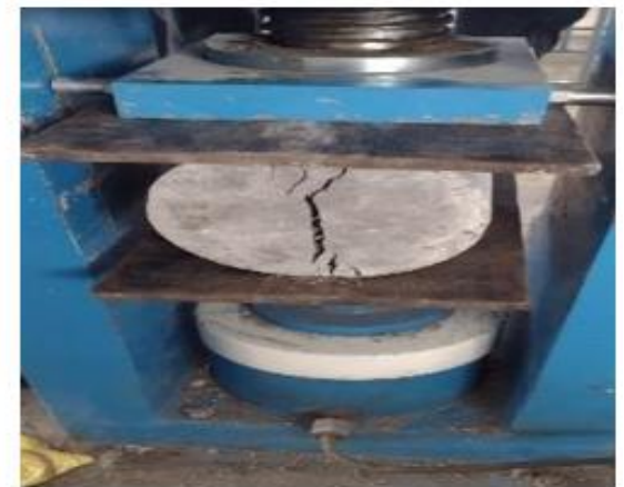
Figure 4: Testing of the cylinder for split tensile strength
