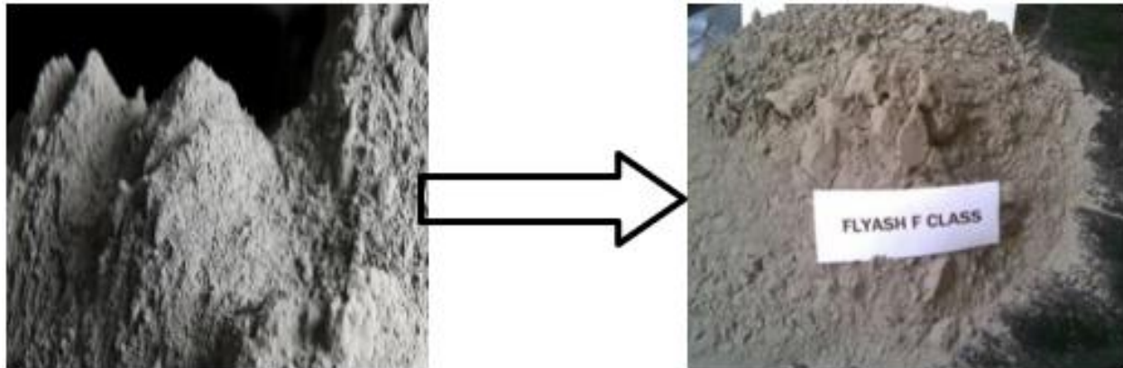
Figure 1: Partial replacement of cement with Class F Fly ash
