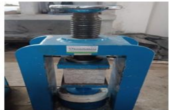
Figure 3: Testing of the cube under direct compression
