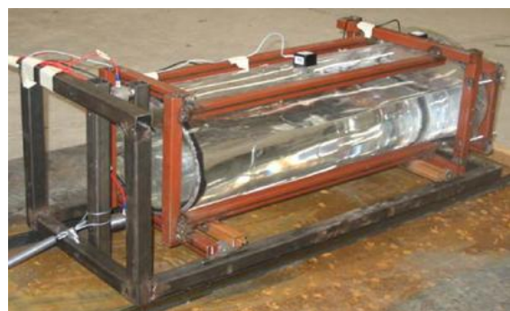
Fig. 12 Scaled experimental test set up used to study the sloshing mechanism [31]
