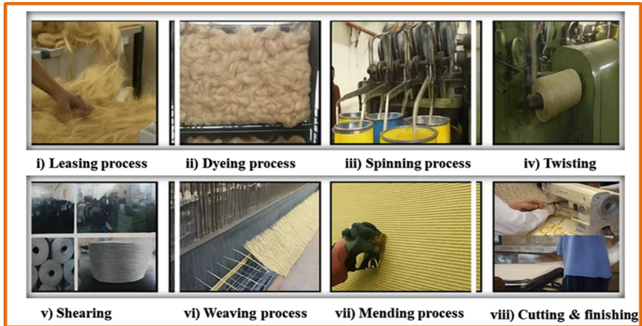
Fig 1: Manufacturing process of hybrid woven
