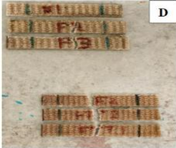
Fig 8: Specimens rupture after Testing a) Tensile b) bending
