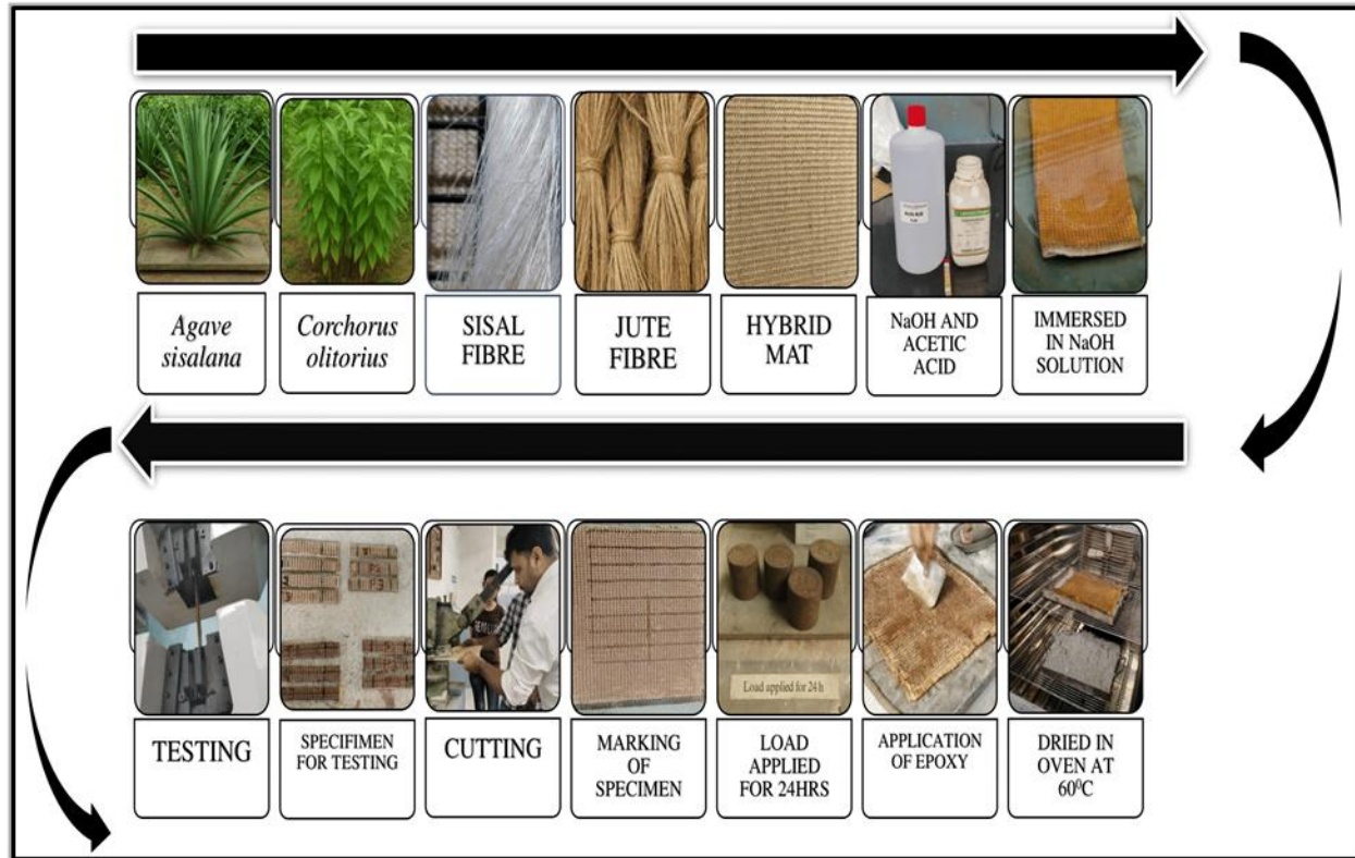
Fig 3: Preparation of HNFRP composite
