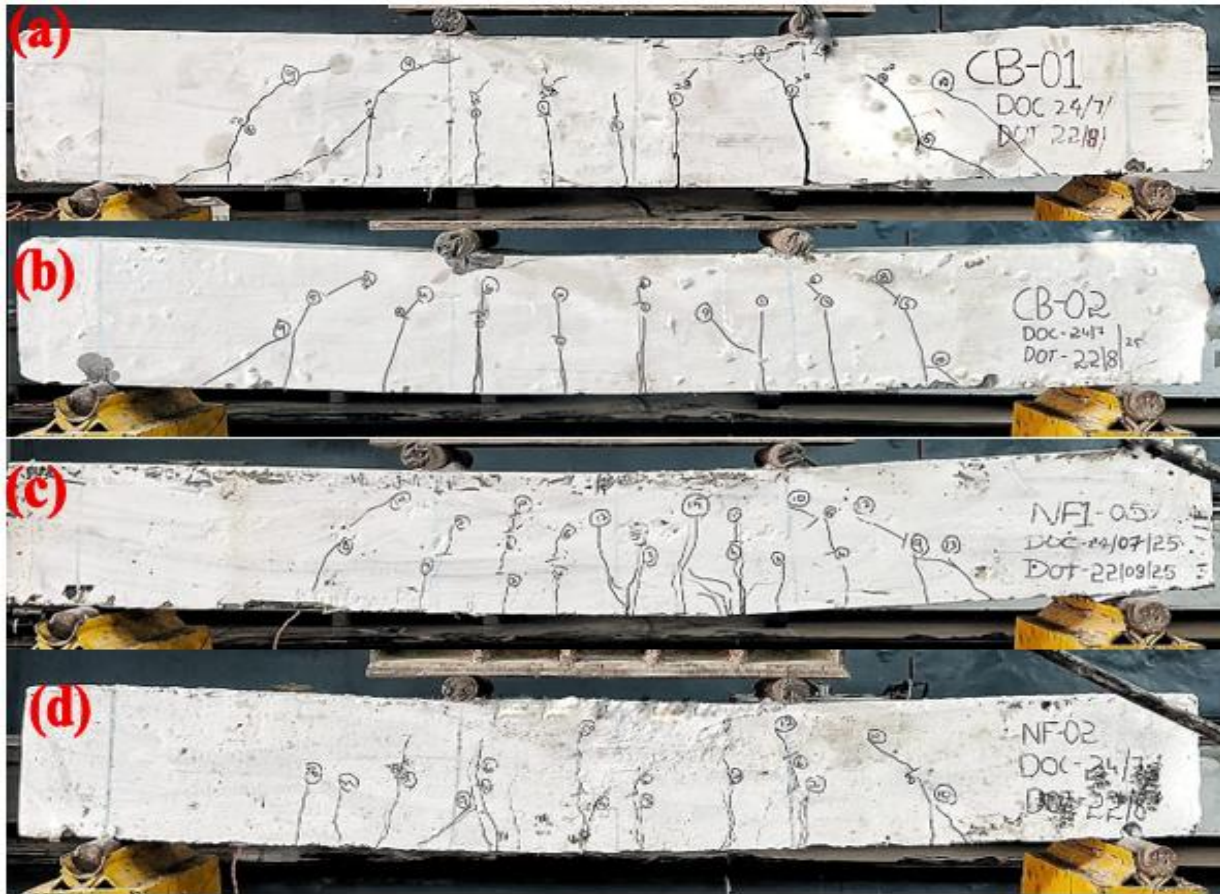
Figure 6: Crack Patterns of RC beams at Ultimate load (CB: Control Beam, NF: Hybrid Natural Fiber RC beam) (a) CB 01 (b) CB 02 (c) NF 01 (d) NF 02
