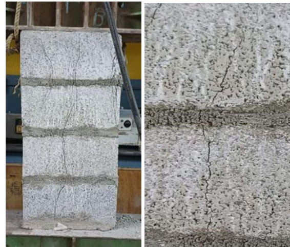
Fig.7 Crushing & Splitting mode of failure of masonry prism specimens
