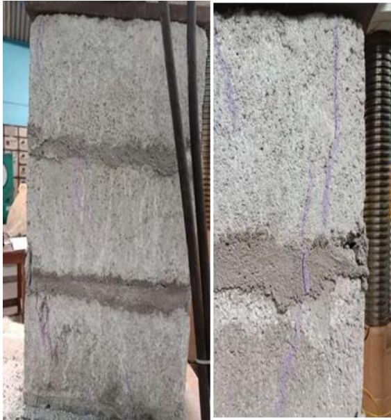
Fig.8 Failure mode of triplet specimen
