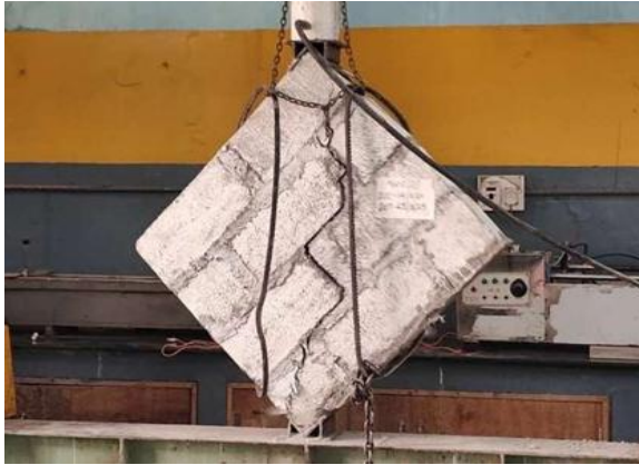
Fig.10 Failure pattern of Diagonal Compression Test
