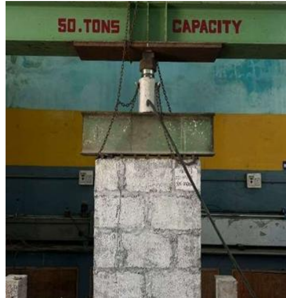
Fig.9 Failure pattern of Compression Test
