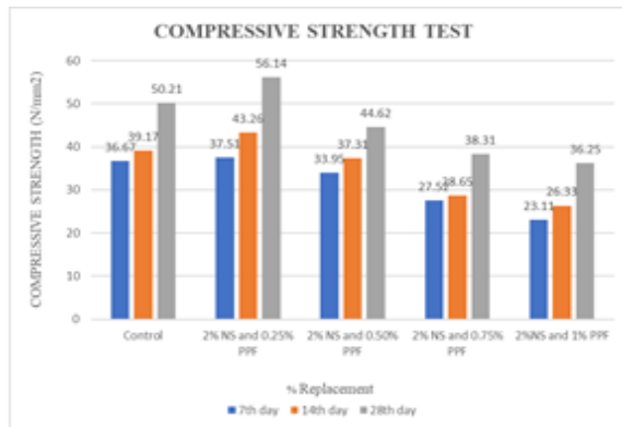
Fig: Compressive-strength graph
