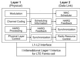
To ensure reliable and scalable communication in LTE femtocell base stations, a modular and standards-compliant Layer 1 (L1) to Layer 2 (L2) interface is essential. The proposed theoretical model presents a structured design that bridges the physical (PHY) and MAC layers while adhering to 3GPP specifications for interoperability and performance. This model is designed to support both traditional LTE deployments
