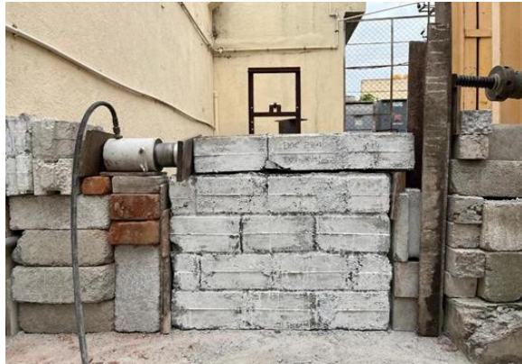
Figure 6. Mode of failure of interlocking block masonry wall
