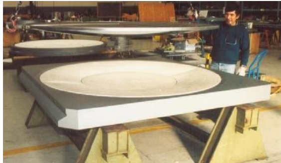
Fig. D Lowering of convex rotational element on Hollow backing plate of 110 MN capacity guided spherical bearing.
