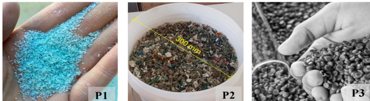
Figure 2. Different forms of plastic waste materials used in permeable concrete: (P1) Plastic powder, (P2) Shredded plastic fibers, and (P3) Plastic pellets.
