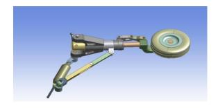
The final assembly accurately represents a retractable main landing gear mechanism suitable for light aircraft or UAV applications.
