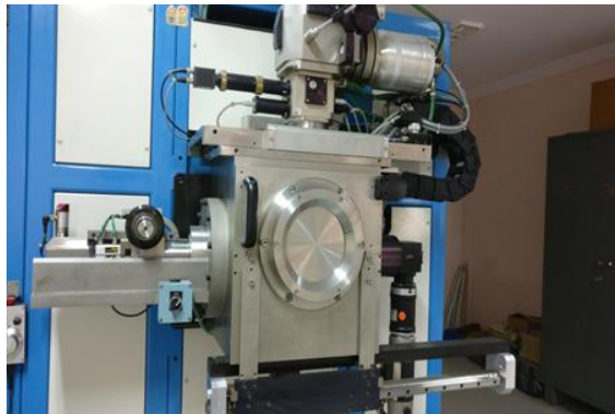
Fig.1 Electron Beam Welding Equipment
