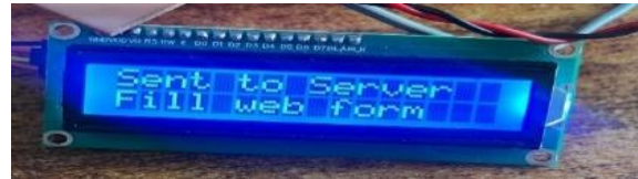
Figure 13: Indicates that the UID is sent to the server for online form completion.
