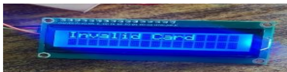
Figure 10: Display when an unauthorized card is scanned.
