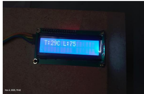
Fig 7: LCD display which shows temperature and level of environment
