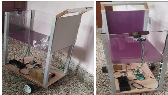
Fig. Pictorial of Smart shopping cart using OpenCV
