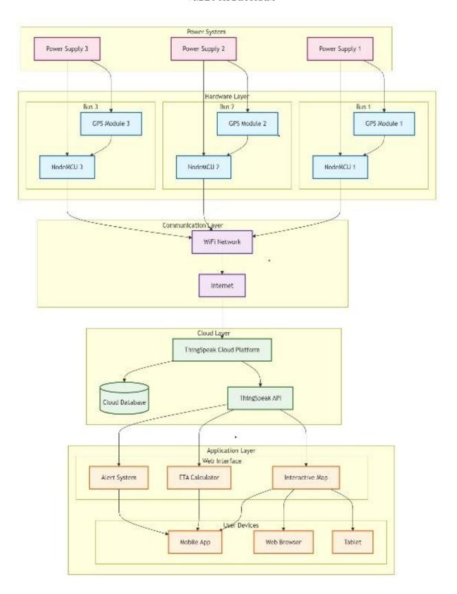
The block diagram of the proposed Real-Time Public Transport Tracking System illustrates the end-to-end flow of data from vehicle-mounted sensing units to the end-user interface through cloud infrastructure. The system architecture is modular, scalable, and IoT-enabled, ensuring reliable real-time tracking of public transport vehicles.
