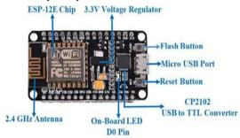
Node MCU can be powered using a Micro USB jack and VIN pin (External Supply Pin). It supports UART, SPI, and I2C interface.
