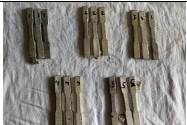
Fig 11. Tensile test specimen before testing
