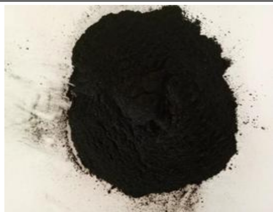
Fig 3. Coconut shell fly ash
