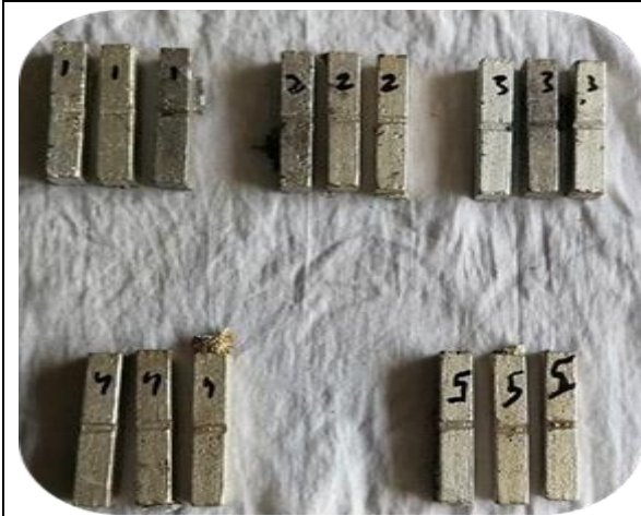
Fig 13. Impact test specimen before testing
