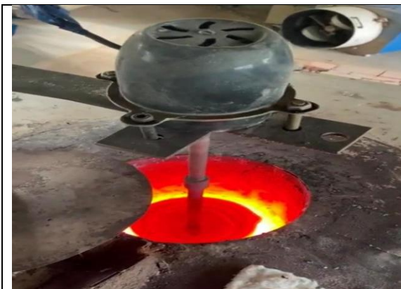
Fig 5. Stir casting setup for synthesizing aluminum 7075 based hybrid composites
