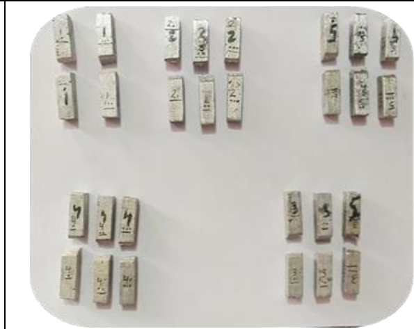
Fig 14. Impact test specimen after testing
