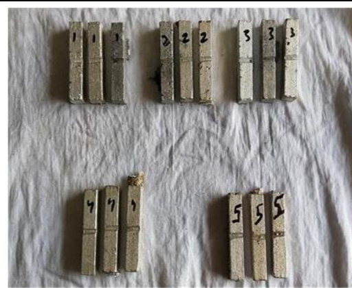
Fig 7. Impact test specimen
