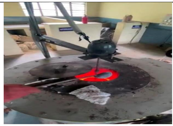
Fig 5. Stir casting setup for synthesizing aluminum 7075 based hybrid composites
