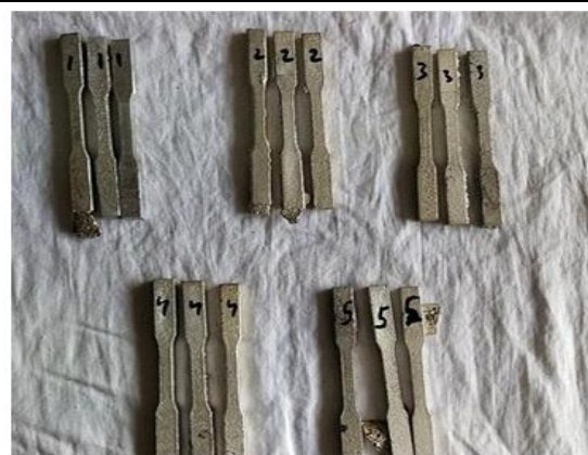
Fig 6. Tensile test specimen
