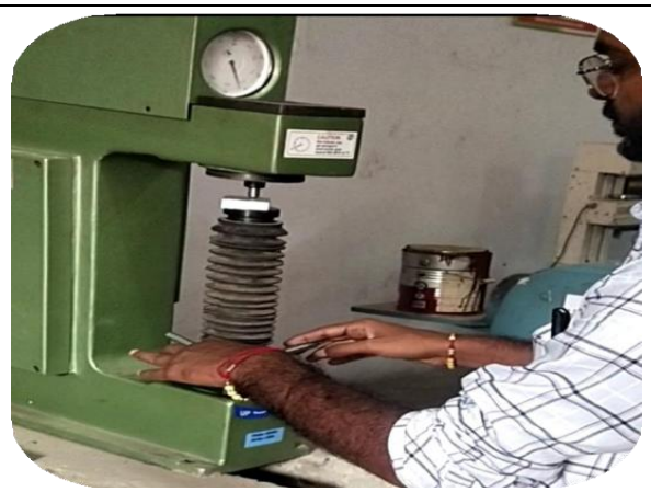
Fig 16. Rockwell hardness testing machine
