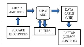
The block diagram illustrates the working of the proposed EOG-based cursor control system. Surface electrodes placed around the eyes capture the electrical potentials generated due to eye movements. These weak EOG signals are amplified using the AD8232 biopotential amplifier to obtain a measurable analog output.
