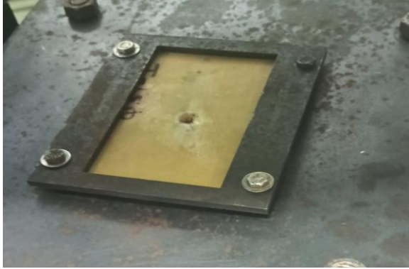
Fig.6 . Quasi static specimen after quasi static testing
