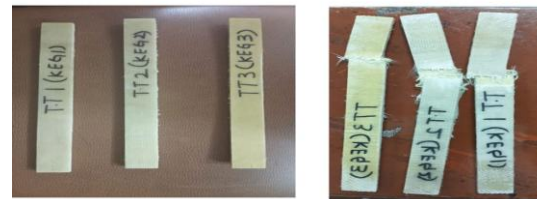
(a) (b) Fig.4 . (a) Tensile test specimens before , (b) Specimens after Tensile Test.
