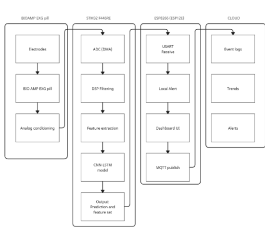
Figure 3: Firmware data flow from acquisition to output.
