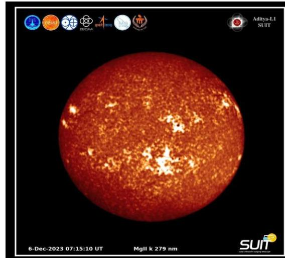
The Solar ultraviolet imaging telescope (SUIT) instrument on board the ADITYA-L1 spacecraft capturing NB3 (Mg II K) showing chromosphere, sunspots, plages and filaments <https://suit.iucaa.in/>
