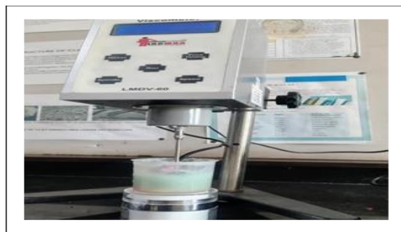
Figure No. 7 Measurement of viscosity using Brookfield viscometer
