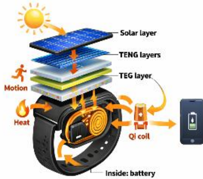
Fig.2 Cross-sectional view of the proposed triple-harvesting wristband showing energy collection layers and wireless charging coil.
