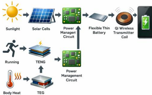
Fig.3 Block diagram of the energy harvesting and wireless charging system in the wristband.
