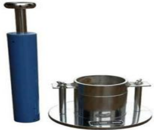
Fig 3.1. Modified Proctor test apparatus
